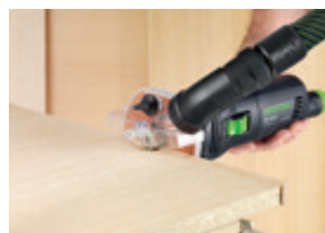
Flush trimming of plastic or solid wood veneer.
